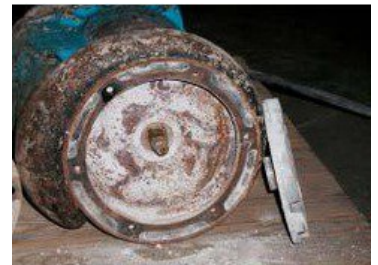
After 11 months of operation (November 2000 till September 2001) the pump did not show any major sign of wear
