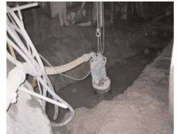
KRS2-100 for sludge pumping
